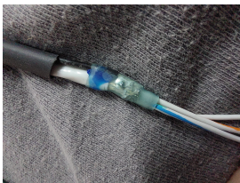
Close up image of the solder sleeve
